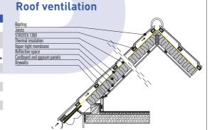
STROTEX 1300 is laid directly on the heat insulation. High vapor--permeability allows penetration of vapor.
